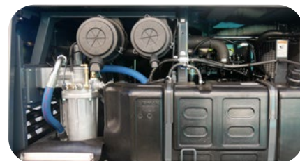
Two heavy-duty air filters with additional safety elements
