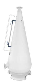
Oxygen cones are used to enter and mix oxygen into bodies of water, particularly in an aqua culture environment. It is used both in closed circuits as well as in the flowing ponds. Water inside the cone provided by circulation pumps is mixed with oxygen supplied from a separate vessel. Maximum pressure that arises does not exceed 2 bar. Oxygen supply pressure must not be higher than 2 bar.
